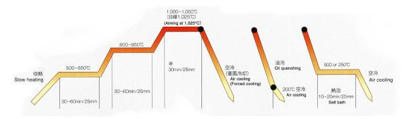
※:加熱保持時間 (Holding time) 雰囲気炉 (Atmosphere-controlled furnace) ......30min/25mm ソルトバス (Salt bath) ·······30min/25mm (浸漬時間 Immersion) 真空炉(Vacuum furnace) ·······40-60min/mm
